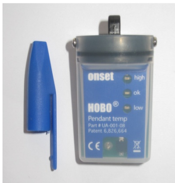
Figure 1: Hobo data logger used to measure indoor air temperature in 292 dwellings in Leicester.
