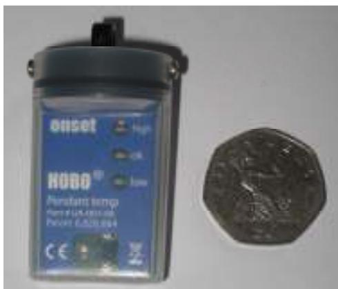
Figure 1 Hobo data logger used to measure air temperature in the living room and main bedroom
