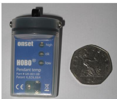
Figure. 1 Hobo data logger used to measure indoor air temperature in 290 dwellings in Leicester City.
